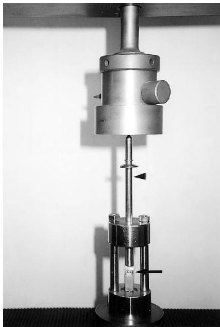
Figure 1 The Instron testing machine with a shearing instrument (arrowhead) resting on a bracket bonded to the crown of the tooth (arrow).
